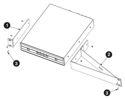
Figure 1. Single Mount (Quad Unit Shown)
